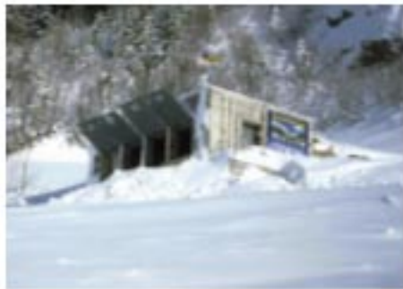
The Swiss Avalanche Institute's scientists climb into this sensor-covered bunker and then trigger an avalanche. As snow and ice crash down upon them by the ton, they calmly collect data to learn more about avalanches
